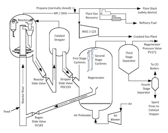
Figure 1: MRC's Catalytic Cracking Unit
